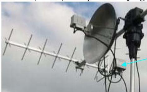
Fig 2:- The 70cm X-Quad attached to the boom with the pre-amp in the correct position,
