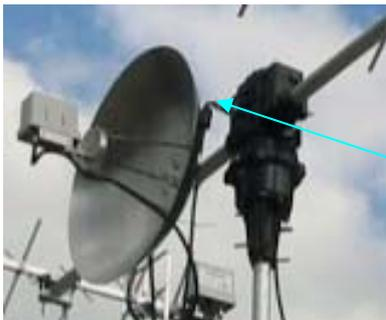
Fig 1:- G3RUH Dish with Down converter installed on “front”/ “north” of rotator assembly.
