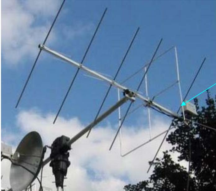
Fig 3:- The 2m X-Quad fitted on the boom relative to the dish and with the pre-amp in the correct position
